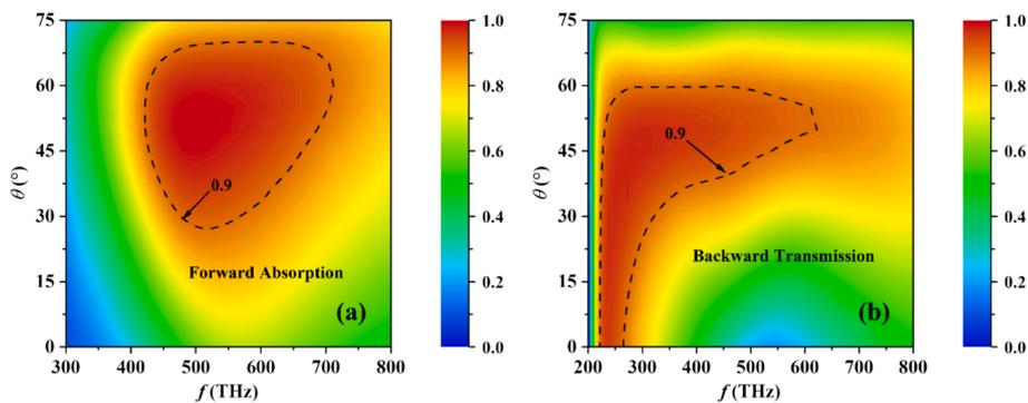
Fig. 8. Absorption and transmission spectra of the SCMPC 2 for different  $\theta$  in both forward and backward propagation directions. (a) Absorption spectra in the forward propagation and (b) transmission spectra in the backward propagation. The ideal absorption and transmission regions are indicated by black dashed lines with a critical value of 0.9.
