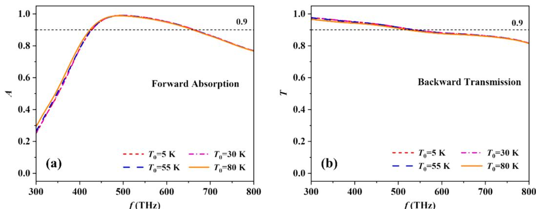
Fig. 9. Effects of different temperatures on (a) forward absorption, and (b) backward transmission.
