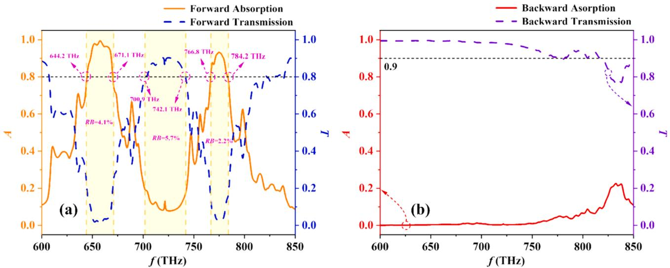
Fig. 4. (a) The absorption-transmission-absorption curves for the SCMPC 1 at forward incidence. (b) Propagation characteristics curves of the SCMPC1 at backward case.
