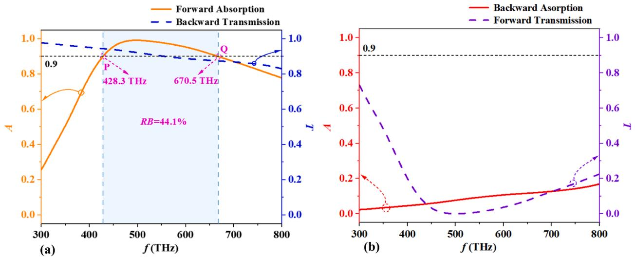
Fig. 7. (a) forward absorption and backward transmission curves and (b) backward absorption and forward transmission curves of the SCMPC 2 when  $T_0 = 50$  K. Points P and Q indicate the intersection of absorption curves with  $A=0.9$ , and the broadband AAT region is indicated by the light blue shaded box.
