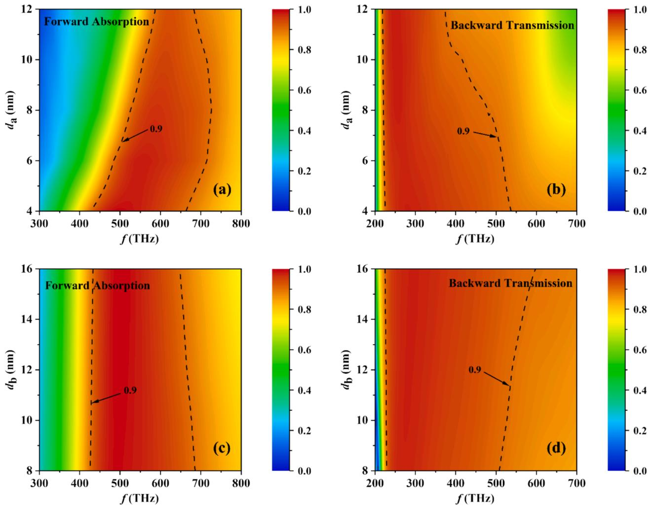
**Fig. 10.** The forward absorption and backward transmission properties of the SCMPC 2 about the thicknesses of the metal layer A and the SC layer B. Effects of  $d_a$  on (a) forward-propagating absorption spectra and (b) backward-propagating transmission spectra. Effects of  $d_b$  on (c) the forward-propagating absorption spectra and (d) the backward-propagating transmission spectra. The ideal absorption and transmission areas are indicated by black dashed lines with a critical value of 0.9.
