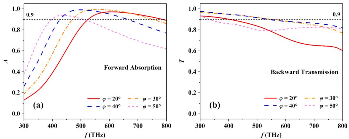
**Fig. 11.** Effects of the inclination angle  $\varphi$  on (a) forward absorption, and (b) backward transmission.
