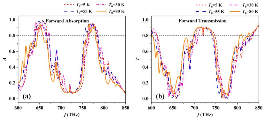
Fig. 6. Effects of different temperatures  $T_0$  on (a) forward absorption, and (b) forward transmission of the double-band rasorber phenomenon of the SCMPC 1.
