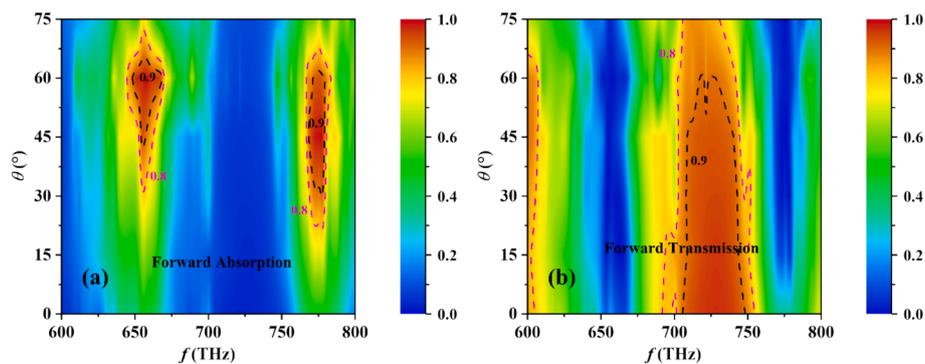
Fig. 5. Effects of variation of incident angle  $\theta$  on (a) forward absorption, and (b) forward transmission of double-band rasorber phenomenon of the SCMPC 1.
