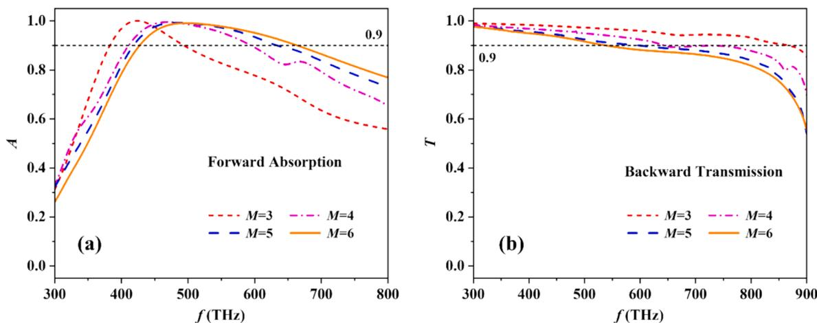
Fig. 12. Absorption and transmission curves in relation to stacking numbers  $M$  of the SCMPC 2. (a) Forward absorption curves as a function of  $M$ , and (b) the backward transmission curves as a function of  $M$ .
