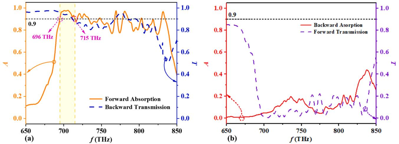
Fig. 3. For the TM modes, (a) forward absorption and backward transmission curves and (b) backward absorption and forward transmission curves of the SCMPC 1.
